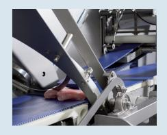
Changing the angle is fast and easy without the use of tools. The optimum gap between the infeed and outfeed belt is adjusted automatically (patent pending).
